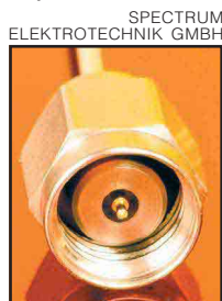
Figure 9—A close-up photo of the 1.85 mm male connector. Anritsu calls this the “V” connector.
