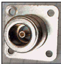
Figure 3—A female N connector. This one is intended to be chassis mounted.
